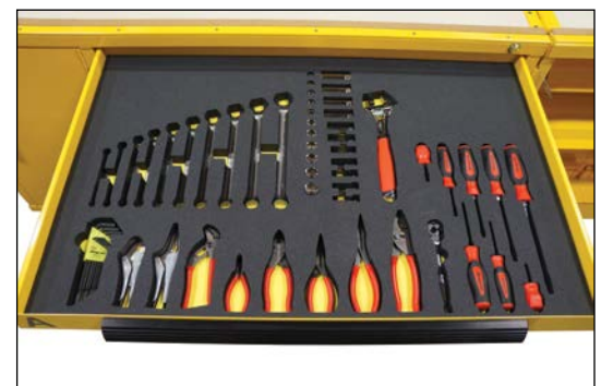
Shadow boxed two color tool control foam
