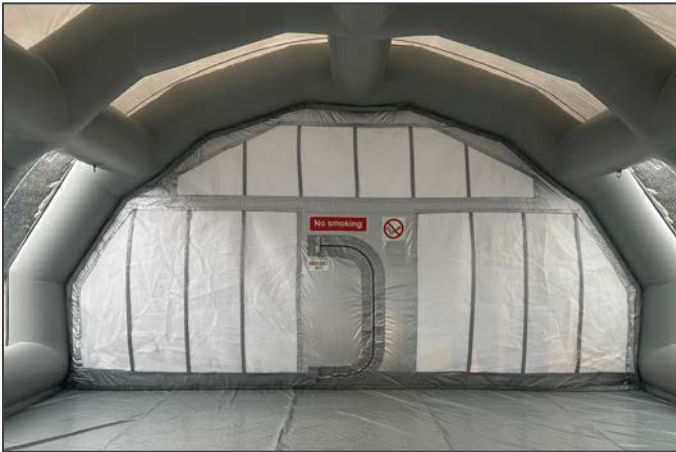
Filtered air enters booth at the rear
