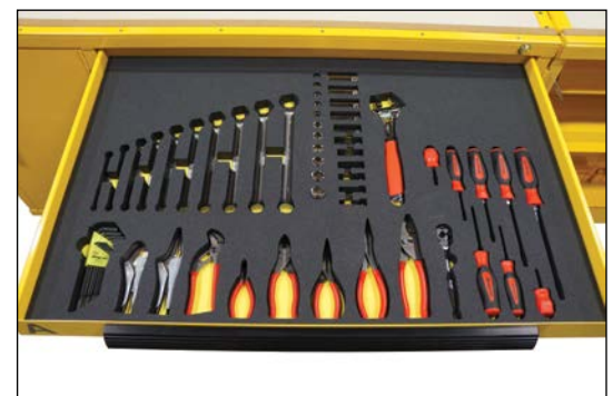
Shadow boxed two color tool control foam
