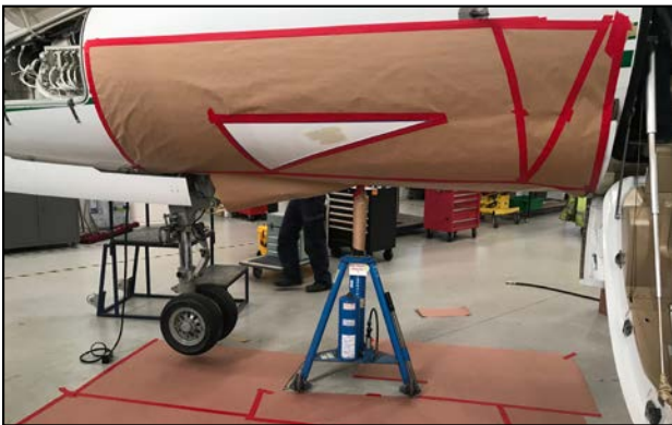
Protect the floor and mask aircraft with rosin paper.
