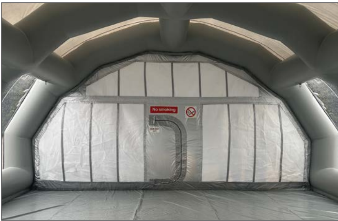
Filtered air enters booth at the rear
